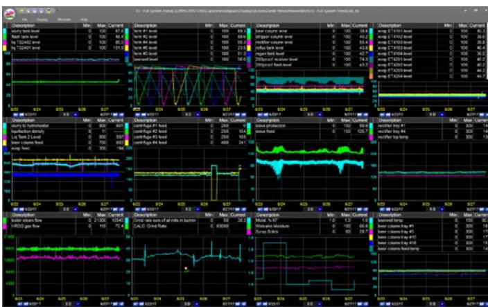
Overview of key trends from the entire plant, from many different sources, including DCS and Lab data.
